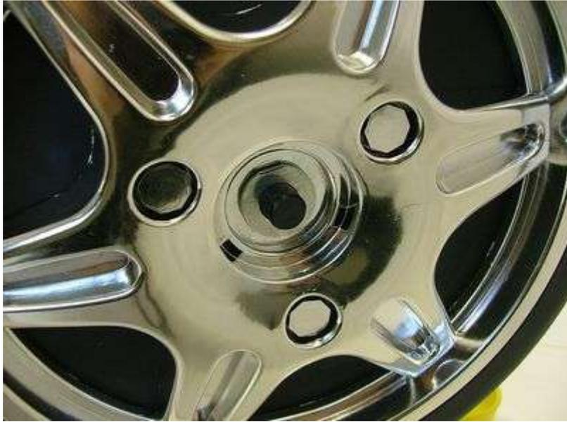
Then to finally fit the wheel in place, have one last check that everything is properly assembled, then push on the wheel securing clip. It will click in to place. Repeat this for both sides. The rear wheels are now secured to the car.
