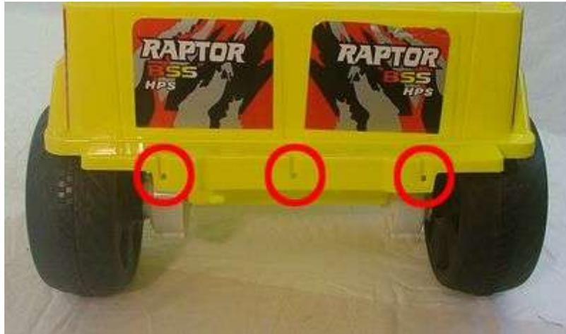
Then place the bumper on the rear of the car, and fix it in place with three screws like this;
