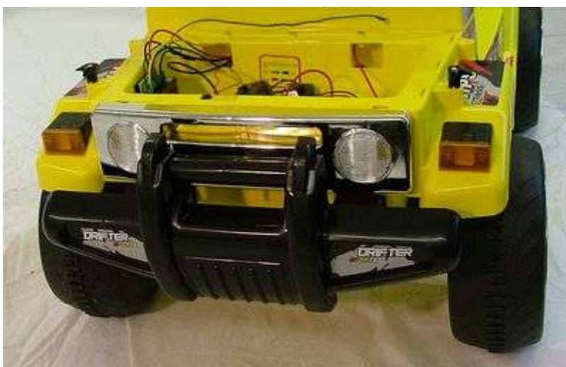
Then, open the bonnet. Inside, you will see where the bumper brackets come out. Fix the brackets in to place inside using two screws for each side.
